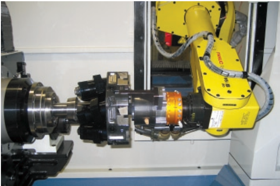
Tooling: Special headstock tooling was designed by ANCA's engineers to hold multiple tools at the same time to reduce load cycle time and increase productivity.
