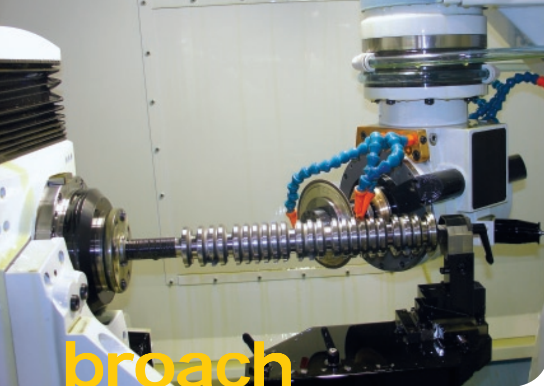
RX7 regrinding a cylindrical broach which is held between centres for total precision.
