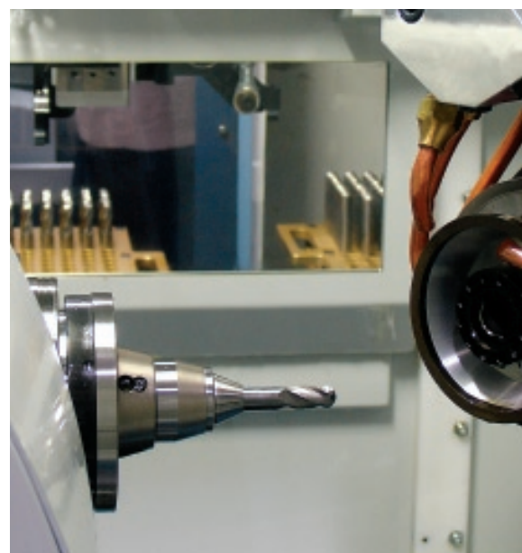
Windows built into the loader ensure full view of its operation from the front of the MX7 machine.
