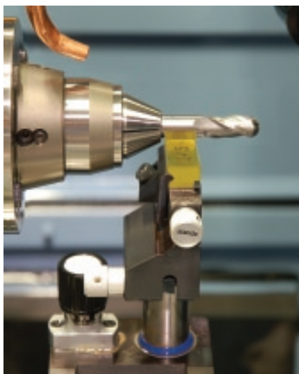
The micro pop-up steady offers optimum tool support and setting control providing vertical, axial and yaw adjustment for excellent accuracy.
