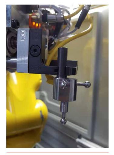
Contact touch probe held in the gripper
