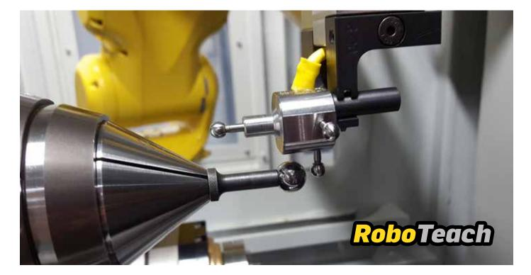
Until now, teaching of the Fanuc Robot (200iD) on RoboMate could be time consuming and labour intensive. In addition to these issues, the accuracy of this task could vary depending on the user conducting the teaching. To solve this problem, ANCA has developed RoboTeach – a product for the automatic teaching of the RoboMate Fanuc 200iD robots on ANCA's MX and TX range of machines.
