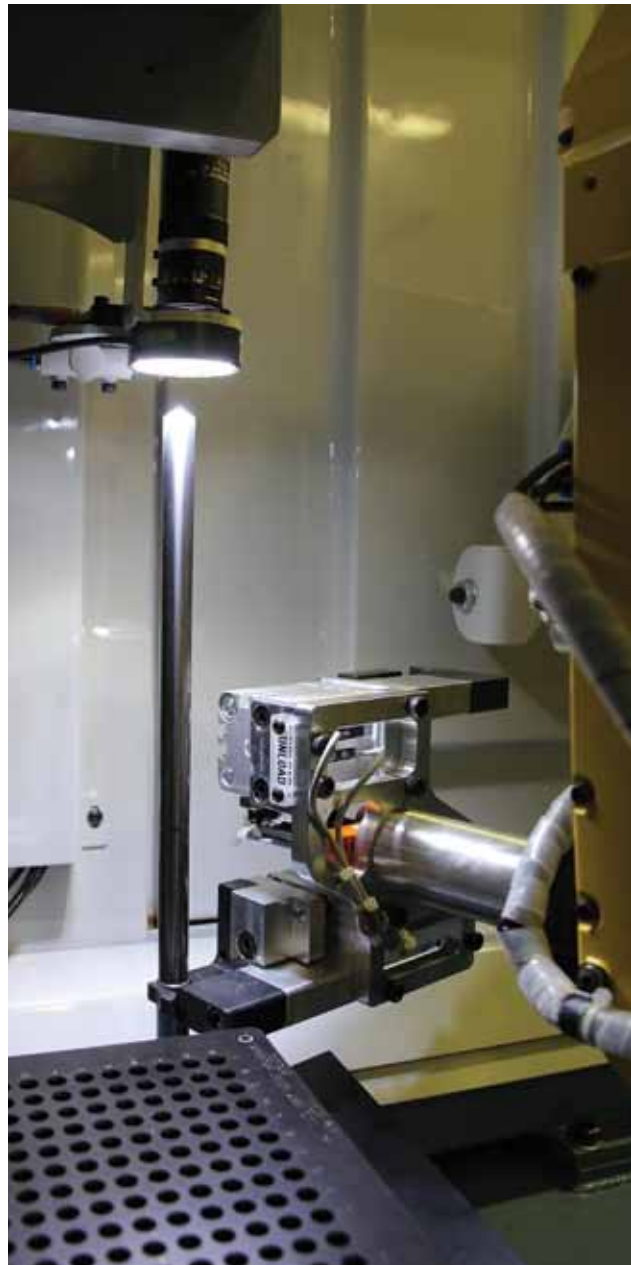
ANCA's Vision system is installed on the RoboMate loader so the verification process is done outside of the grinding cycle.
