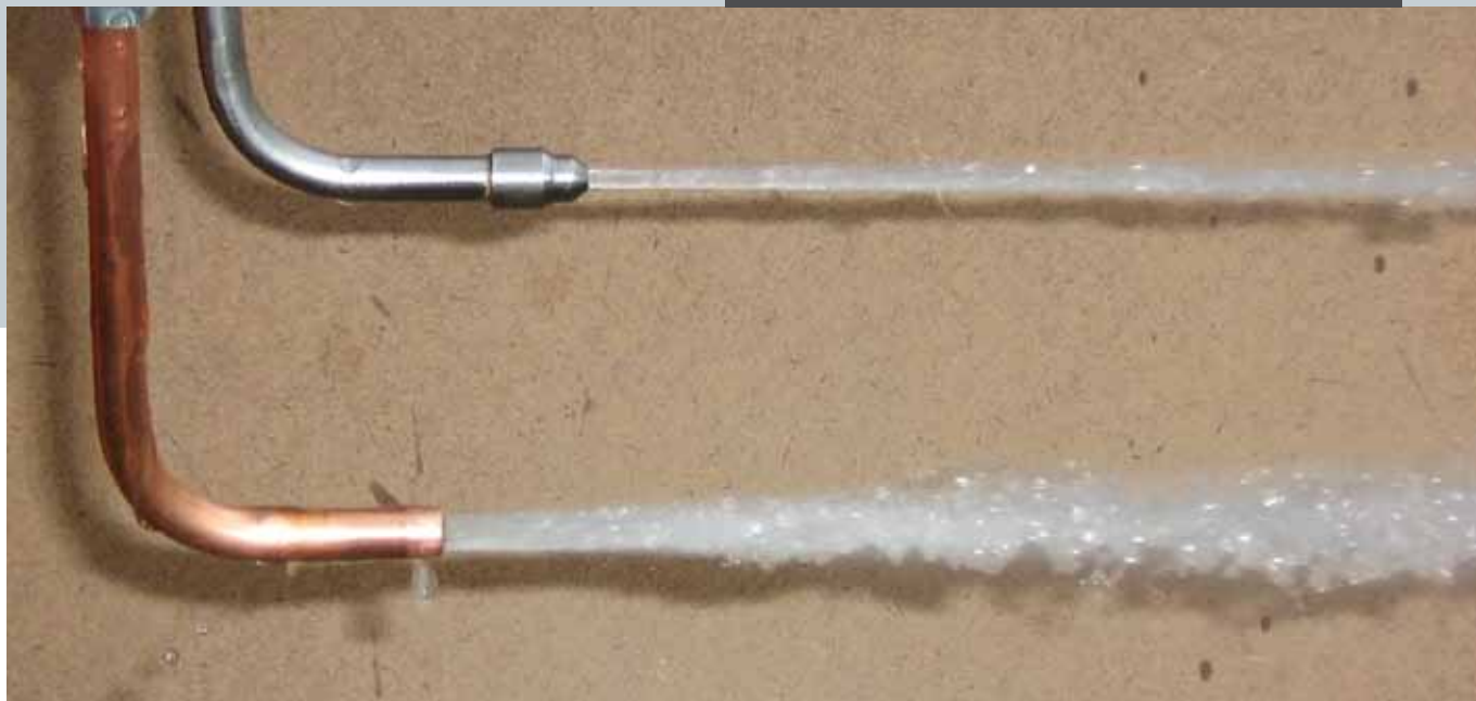
A comparison between a coherent-jet nozzle and an open tube nozzle with water at 120 psi.
