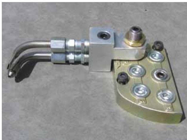
A close-up of a TX7 coolant manifold fitted with a fluting nozzle system matched to the wheel angle.
