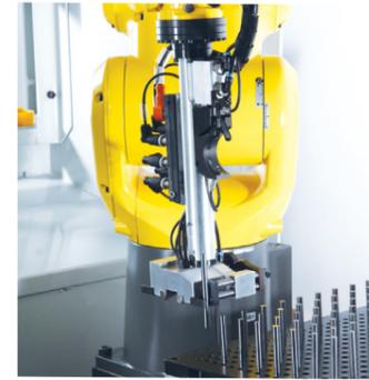
The Fanuc Robot Loader is a versatile automation solution that is located completely within the FX Linear machine. It provides automatic tool loading, enabling extended periods of unmanned operation, for maximised productivity.
