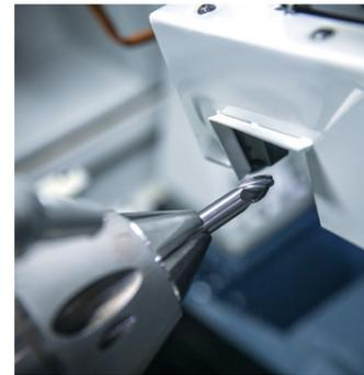
The LaserUltra system provides accurate and repeatable measurement of tools inside the machine. The LaserUltra can automatically measure OD, run-out, EOT, ball nose and corner radius profile tools. An air blast unit on the laser ensures that coolant or contaminants do not interfere with the measurement process.
