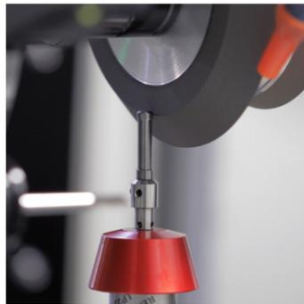
The auto wheel pack qualification probe is used to accurately measure grinding wheels inside the machine. The Wheel Probe uses a Renishaw probe to qualify the wheel pack. It is possible to measure the front surface location, back surface location, wheel diameter and toroid radius of a grinding wheel. It eliminates the need for operator intervention which ensures consistent measurement results.
