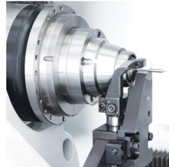
MicroPlus provides less than 3 micron tool runout. It is ANCA's #1 high accuracy work holding and tool support system. The MicroPlus system consists of the Flexi-Chuck assembly for workholding, and the Overhead Top Clamp Assembly (OTC) for tool support. The Flexi-Chuck clamps and rotates the tool. The patented design allows the tool and the internal components to move independently of each other, minimising any misalignment.
