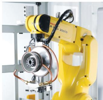
Used in conjunction with the Robot Loader. 6 wheel packs and coolant manifolds are loaded together, stored on a frame next to the robot. A docking station allows the wheel pack to be located close to the wheel spindle for fast wheel change cycle times. The wheel changer is totally contained within the FX7 canopy.
